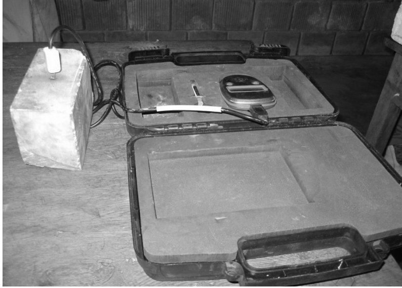
Fig. 3: KD2 probe in a drilled hole inside a sample slab.
