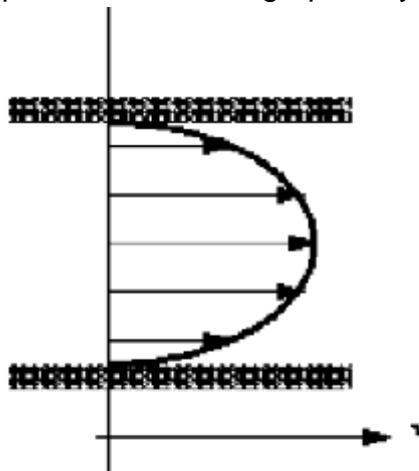
**Figure 11: Velocity profile in a pipe**
