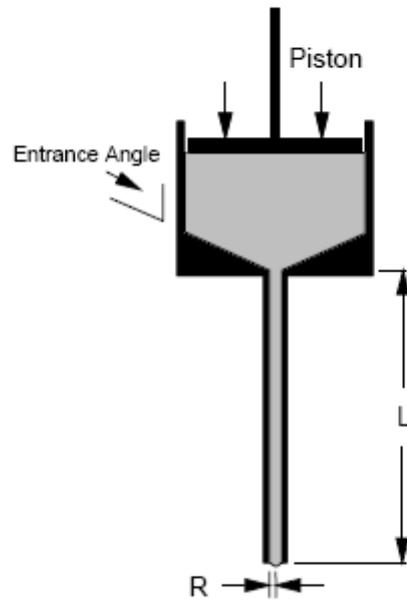
**Figure 9: High pressure capillary viscometer.**
