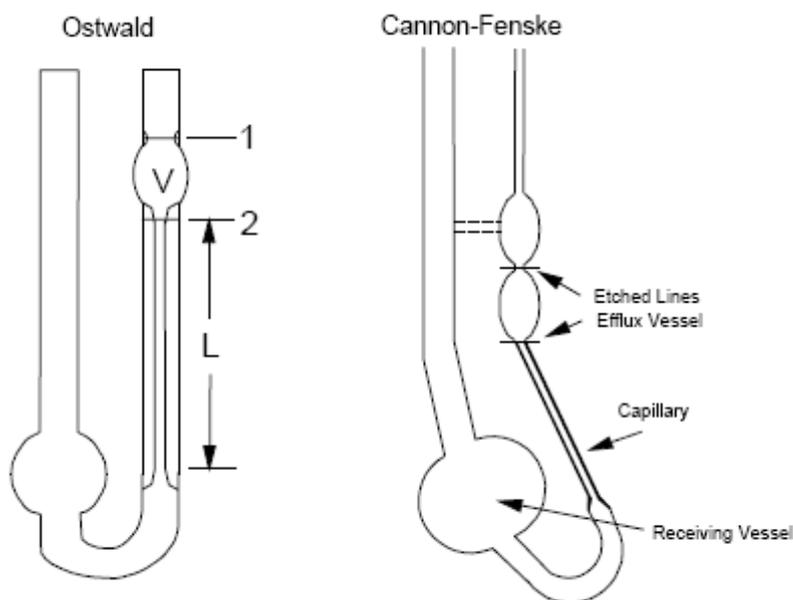
**Figure 8: Ostwald and Canon-Fenske glass capillary (U-tube) viscometers**
