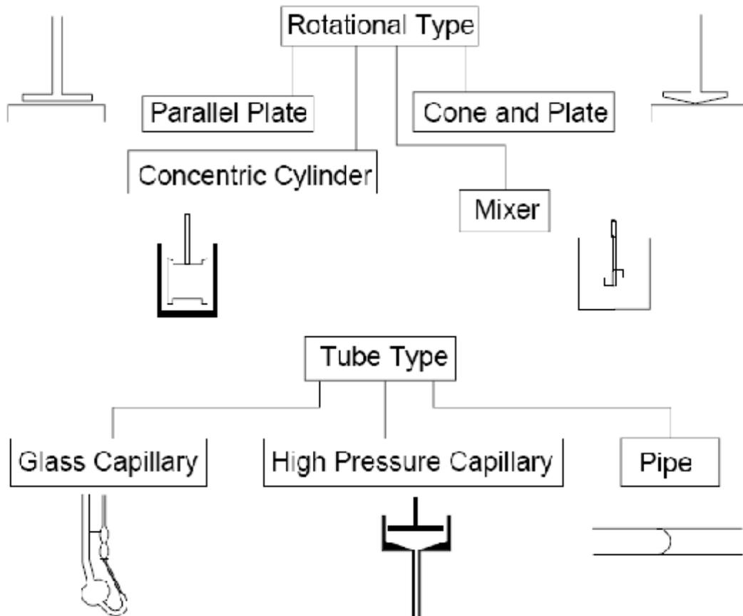
**Figure 7: Common rheological instruments divided into two major categories: rotational and tube type.**
