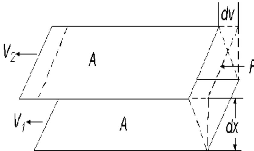
**Figure 1: Isaac Newton's model for viscosity**
