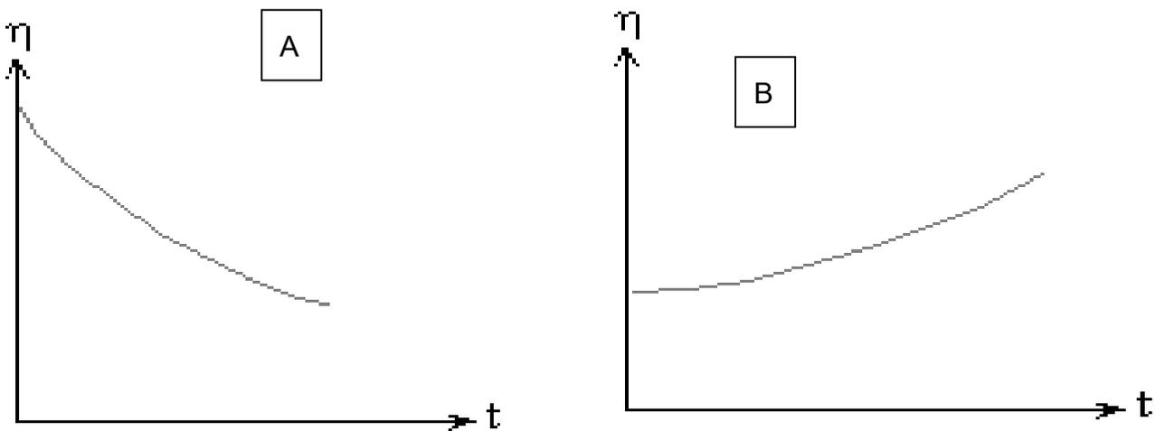
**Figure 6: Graphical representation of (A) Thixotropic Fluids (B) Rheopexy fluids**
