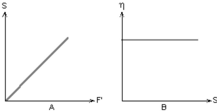
**Figure 2: Graphical representation of Newtonian Fluids (A, shear stress/shear rate; B, viscosity/shear rate)**
