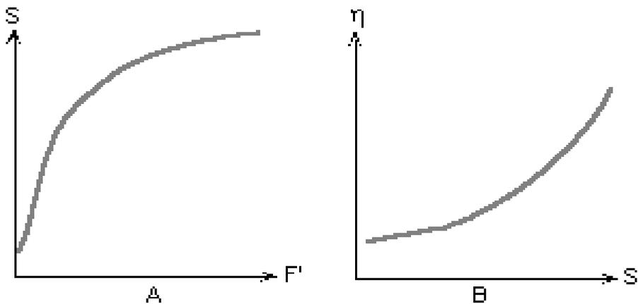
**Figure 4: Graphical representation of Dilatant Fluids**
