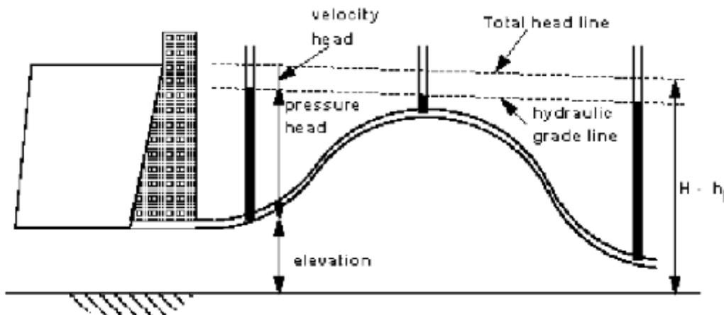
Hydraulic Grade line and Total head lines for a constant diameter pipe with friction
