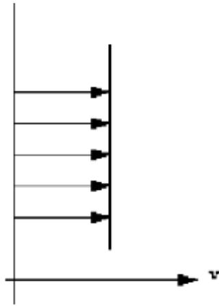
**Figure 12: Velocity profile in uniform flow**
