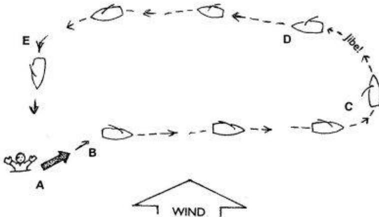
A man overboard (MOB), also called crew overboard (COB) or person overboard (POB), is a very serious boating emergency. Most boating deaths occur after falling overboard. Since you can't trust your engine to start immediately, and since most MOB's don't occur in flat water in calm conditions, you must know how to efficiently turn the boat around and return to and stop beside the person under sail.
