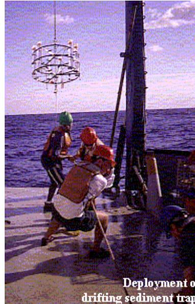
Deployment of drifting sediment trap.
