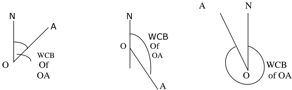
Forward and Back Bearing: with A as the starting station of traverse and the direction of the survey being forward B, the angle between north and AB at A is known as the forward bearing of AB. The angle between north and AB at station B is known as the back bearing of AB, this should differ from the forward bearing by exactly  $180^{\circ}$ .
