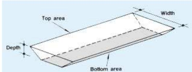
Above all, for precision, prismoidal formula can be used to calculate the volume of soil excavated from pond area (excluding topsoil area):
