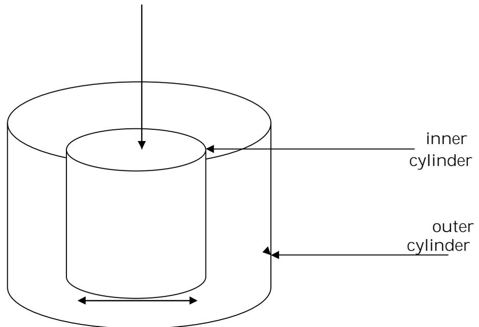
The very infiltration consist of a cylinder driver a fewer continue into the soil to prevent leakage. There are really two cylinder one inside the other and forming two concentric rings on the outside. The inner ring, which is usually 23cm in diameter is the one used to determine infiltration rate. The outer ring 36cm in diameter is meant to reduce the border effects on the inner rings.
