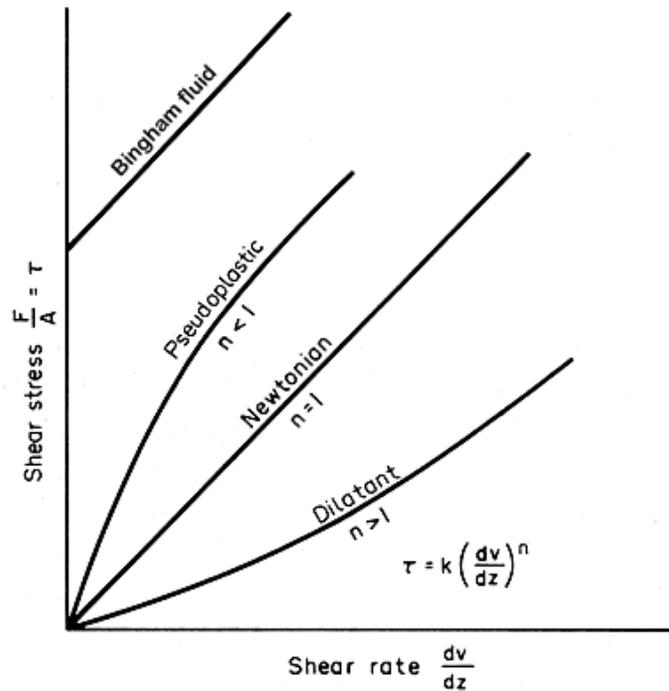
Figure 3.6. Shear stress/shear rate relationships in liquids.
