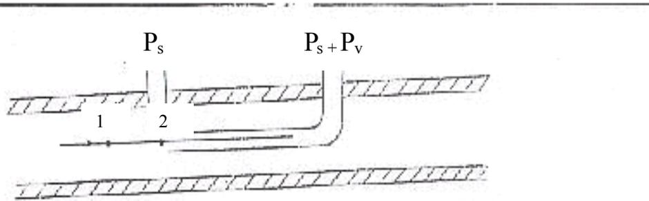
Figure 3: Static and Total Pressure Pitot Tubes
