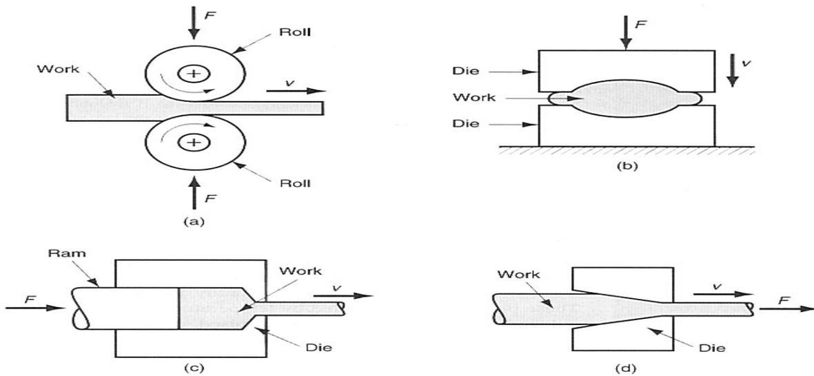
**Figure 2.13: Types of Deformation processes**
