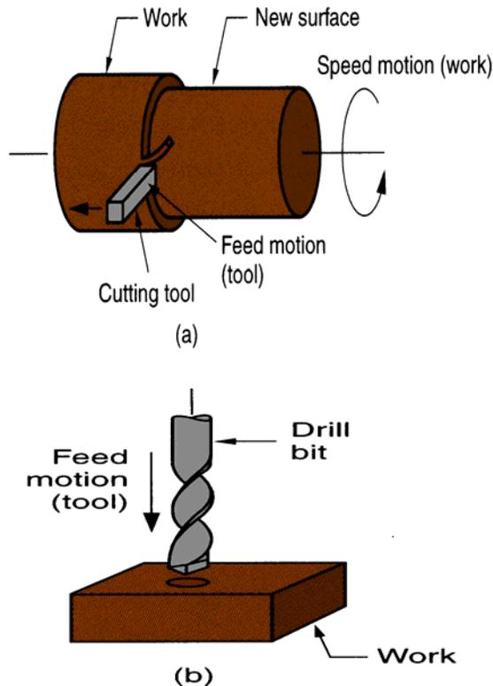
**Figure 2.15: (a) Turning operation (b) Drilling operation**
