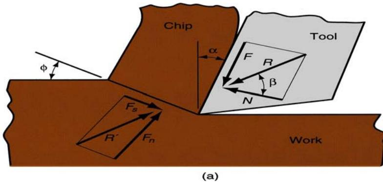
**Figure 3.2: Forces in metal cutting: (a) forces acting on the chip in orthogonal cutting**
