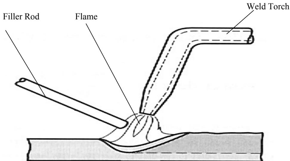
**Figure 5.3: Oxyfuel gas welding operation.**
