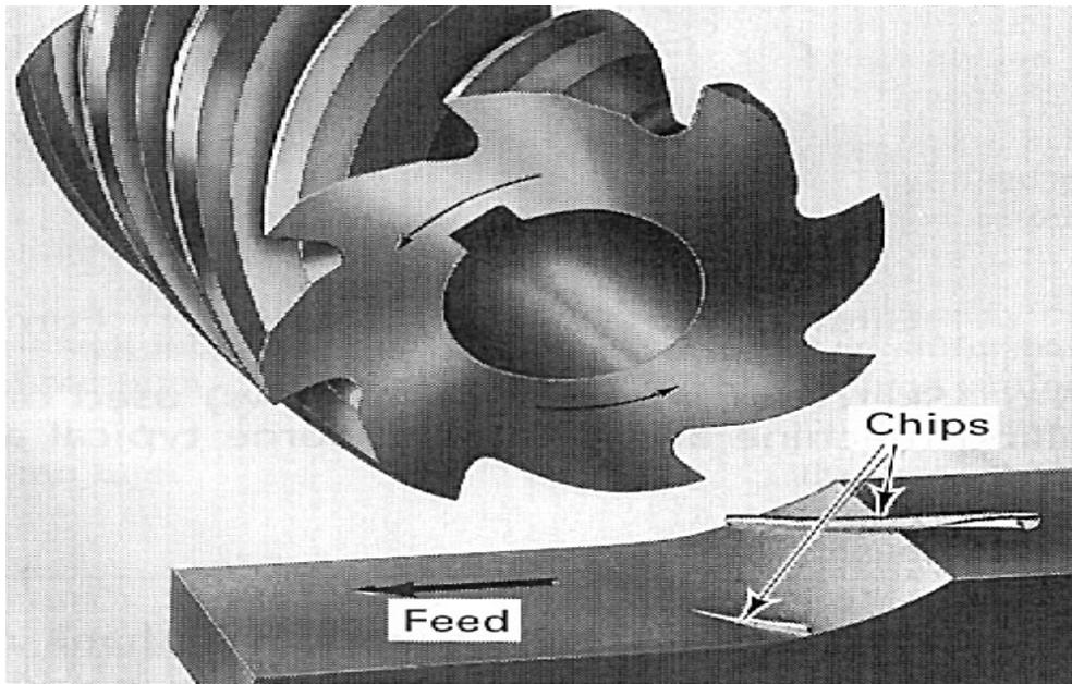
**Figure 2.20: Milling operation.**
