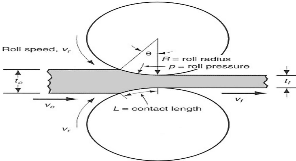
**Figure 2.12: Flat rolling process**
