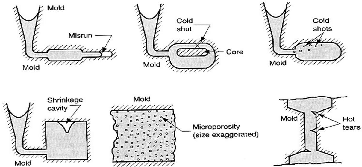
**Figure 2.9: Some defects of casting**
