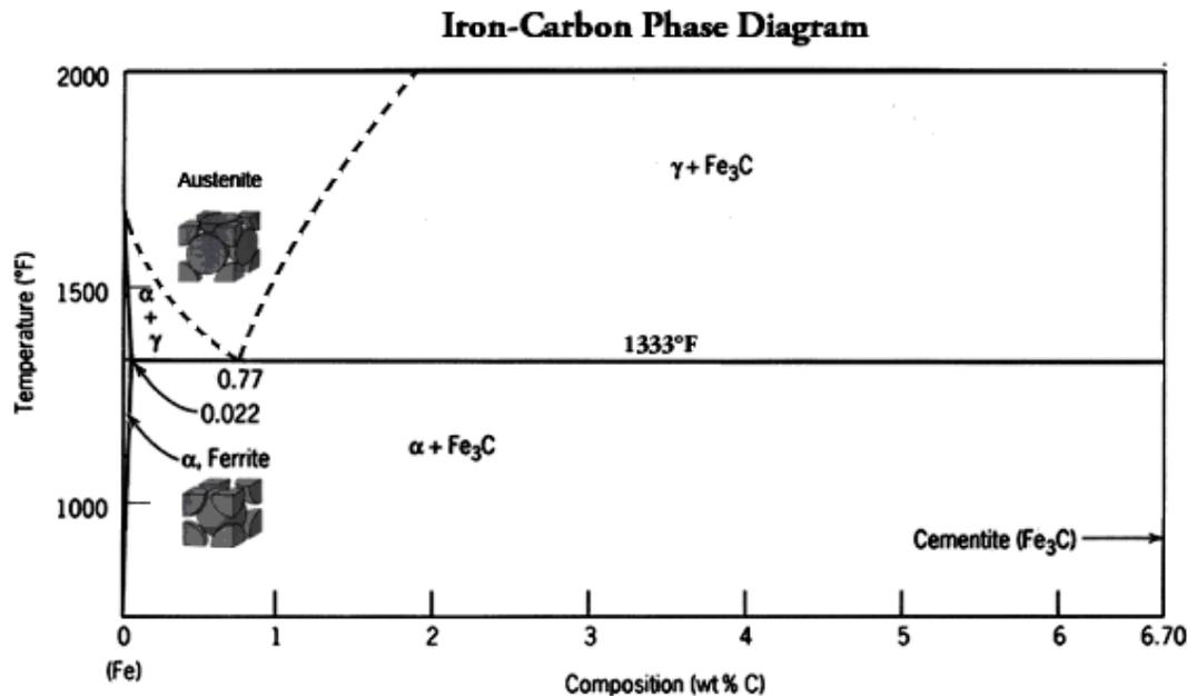
**Figure 6.1: Iron-Carbon Phase Diagram**
