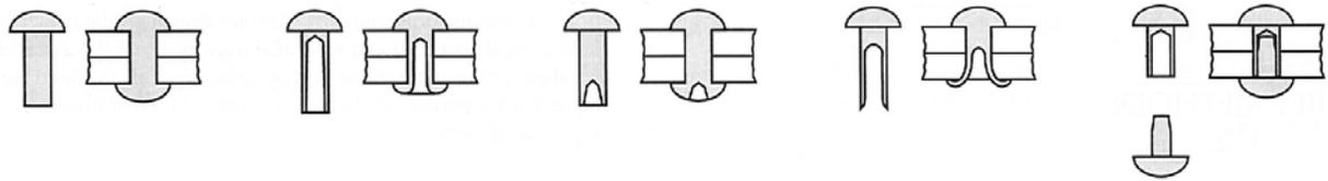
Solid Rivet      Tubular Rivet      Semitubular Rivet      Bifurcated Rivet      Compression Rivet
