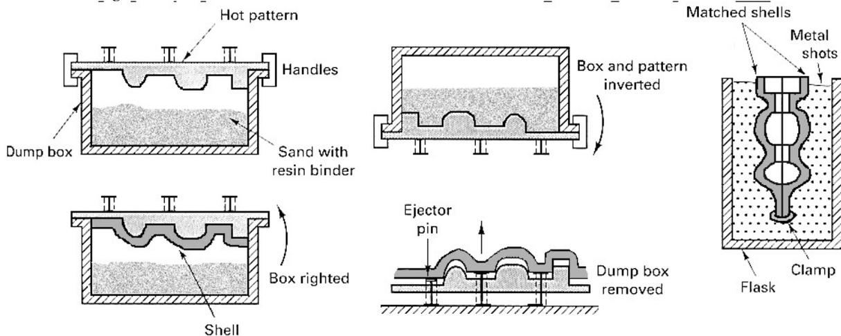
Figure 2.4: Steps in shell moulding
