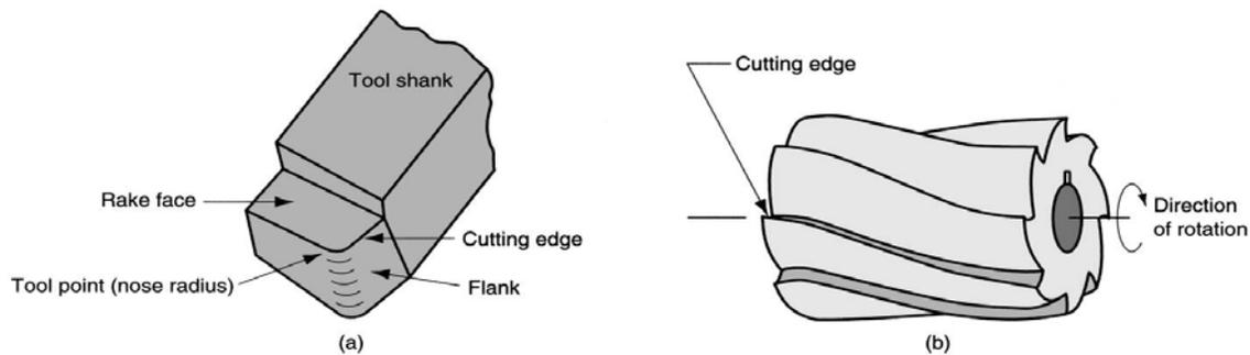
**Figure 2.20: (a) A single-point tool showing rake face, flank, and tool point; and (b) a helical milling cutter, representative of tools with multiple cutting edges.**
