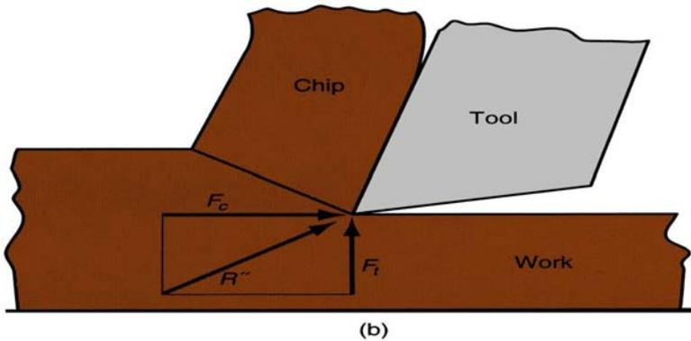
**Figure 3.3: Forces in metal cutting: (b) forces acting on the tool that can be measured**
