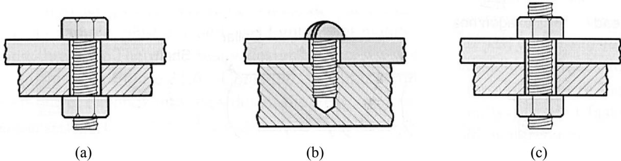
**Figure 5.1: Typical assemblies using (a) bolt and nut, (b) screw and (c) stud and nut.**
