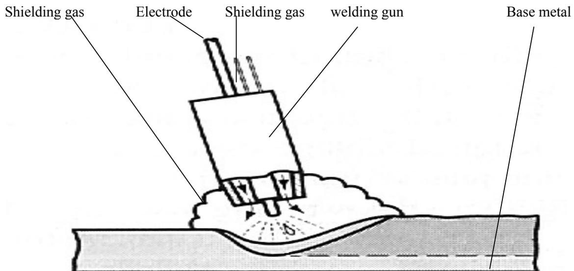
**Figure 5.7: Gas metal arc welding operation.**
