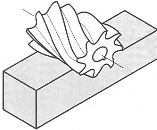
**Figure 2.21: Peripheral slab milling operation**
