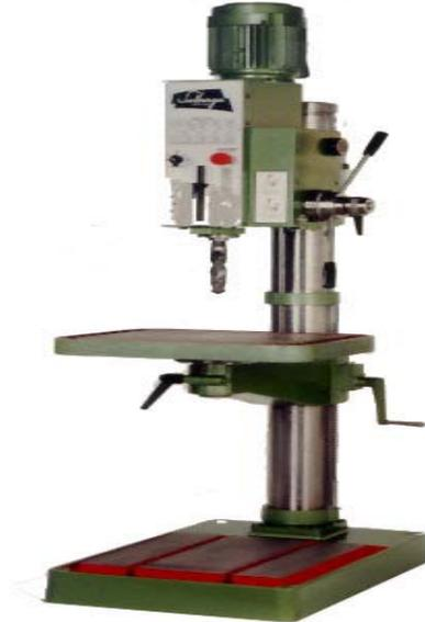
**Figure 2.26: Drilling Machine**
