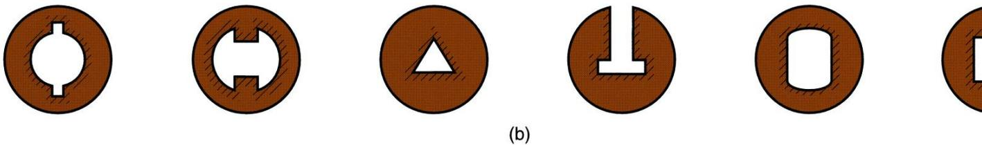
**Figure 2.29: Internal Shapes cut by broaching**
