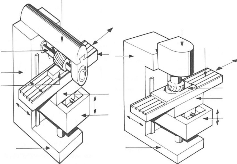
**Figure 2.25:** Two basic types of column-and-knee milling machines, (Left) horizontal, and (Right) vertical.
