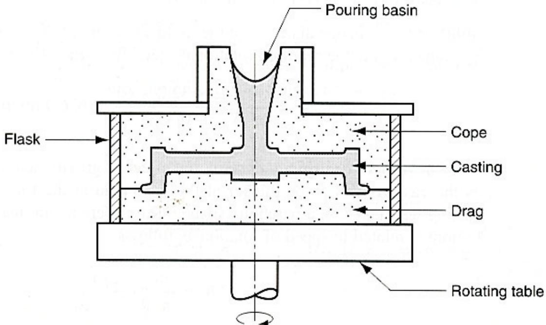
**Figure 2.8: Semi-centrifugal casting**
