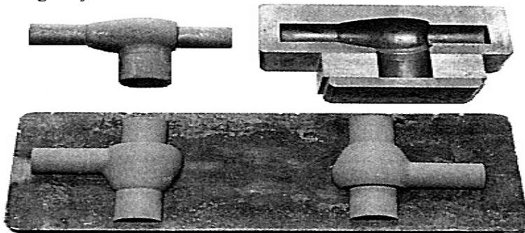
Figure 2.3: Cores used in casting
