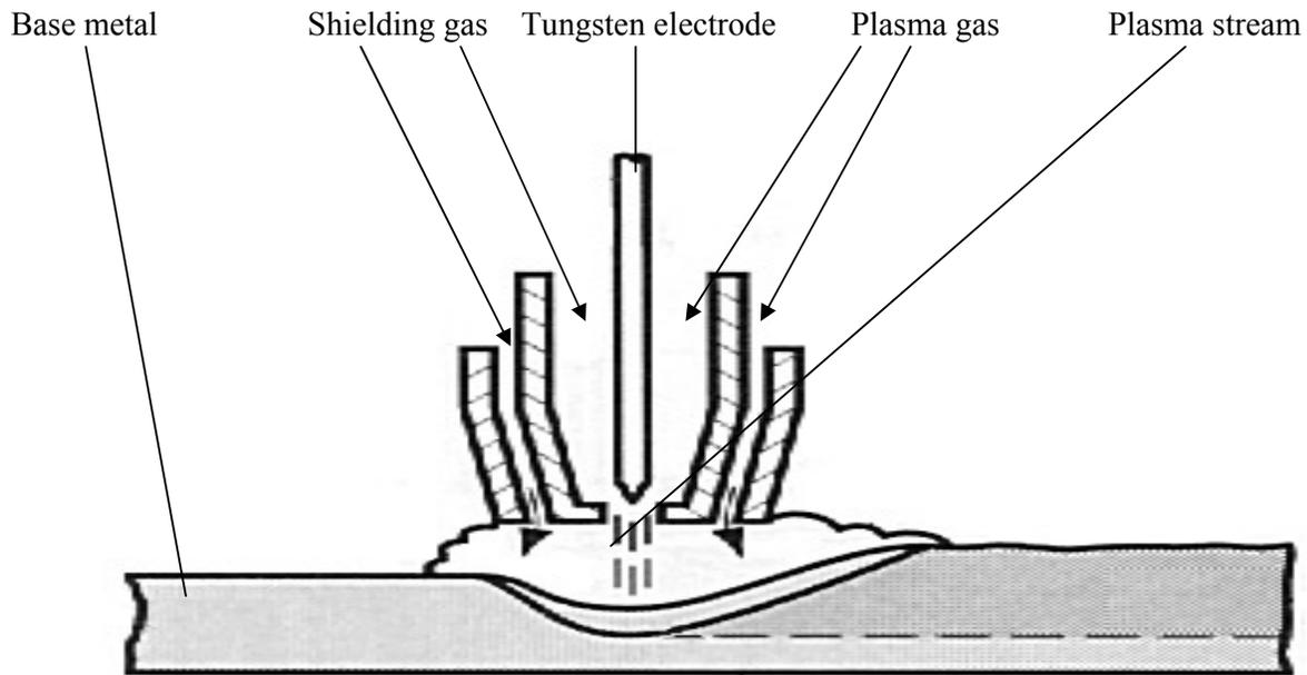
**Figure 5.9: Plasma Arc Welding**
