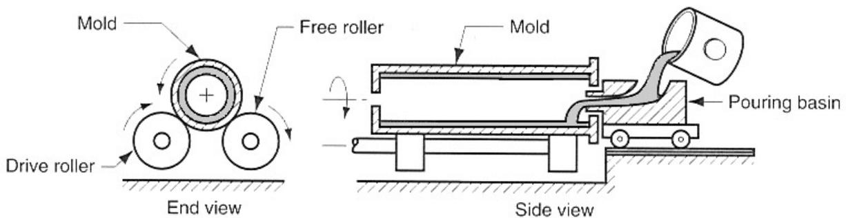
**Figure 2.7: True horizontal centrifugal casting**
