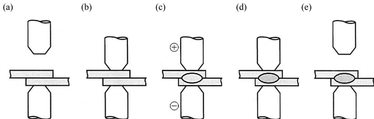
**Figure 5.10: Steps in a spot welding cycle: (a) parts inserted between open electrodes, (b) electrodes close and force is applied, (c) weld time (current is switched), (d) current is turned off but force is maintained, and (e) electrodes are opened, and the welded assembly is removed.**
