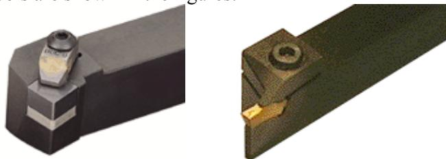
Cutting tool for straight turning
