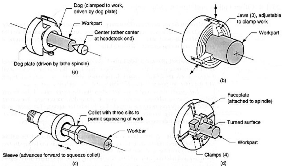
**Figure 2.17: Four Work-holding methods used in lathes:** (a) mounting the work between centres using a dog, (b) three-jaw chuck, (c) collet, and (d) face plate for noncylindrical work parts.
