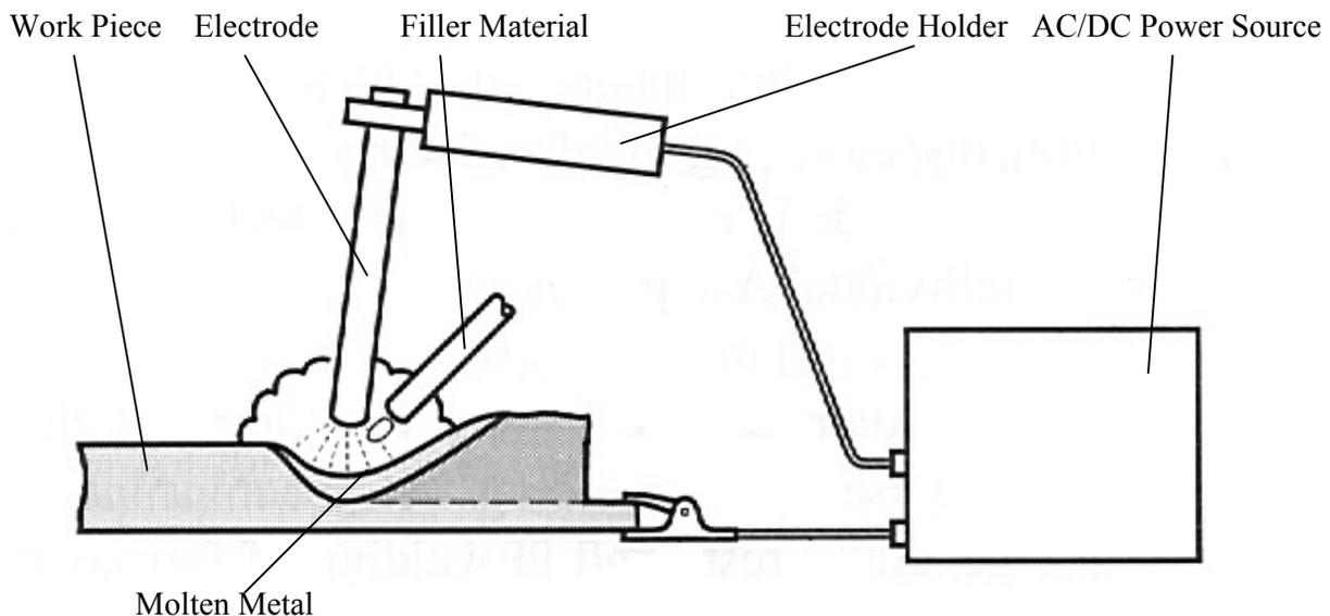
**Figure 5.4: Arc Welding Operation**
