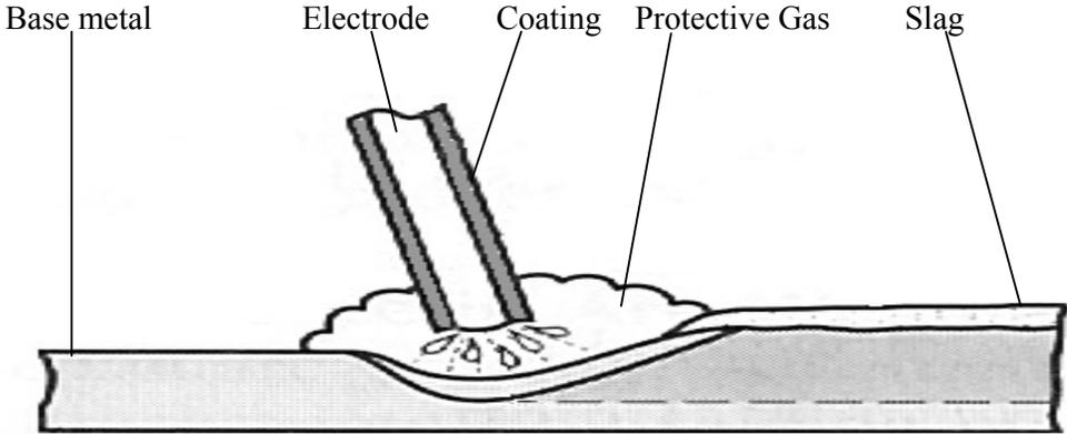
**Figure 5.5: Shielded metal arc welding operation**
