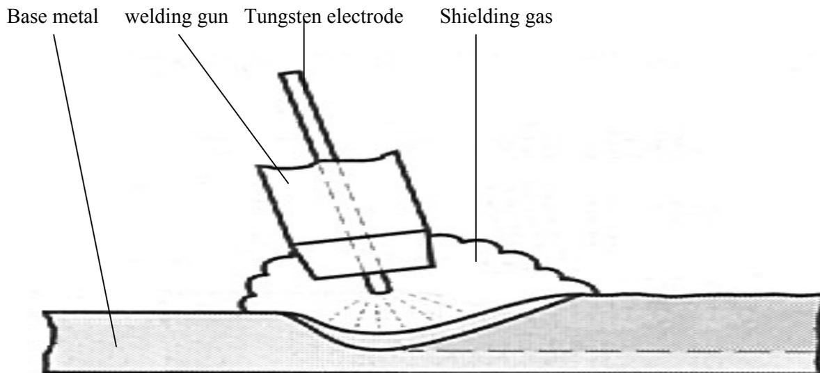
**Figure 5.8: Gas tungsten arc welding operation.**
