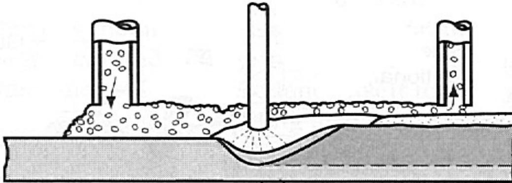
**Figure 5.6: Submerged arc-welding operation.**
