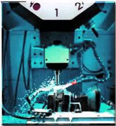
**Figure 3.1: Application of flooding in milling**
