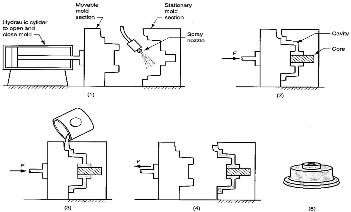
**Figure 2.6: Steps in permanent mould casting:** (1) mould is preheated and coated with lubricant for ease of separation of the casting; (2) cores (if used) are inserted and mould is closed; (3) molten metal is poured into the mould; and (4) mould is open and finished part removed. Finished part is shown in (5)
