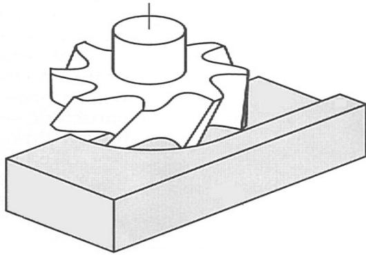
**Figure 2.23: Partial face milling operation.**
