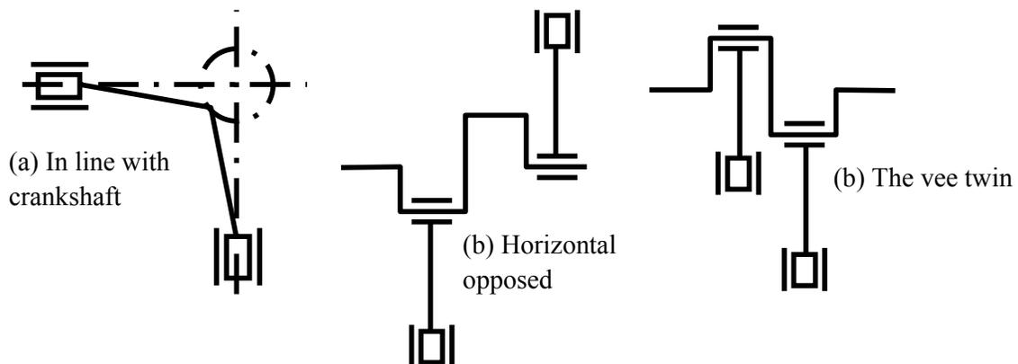
Fig. 1.1: Two cylinder engine
