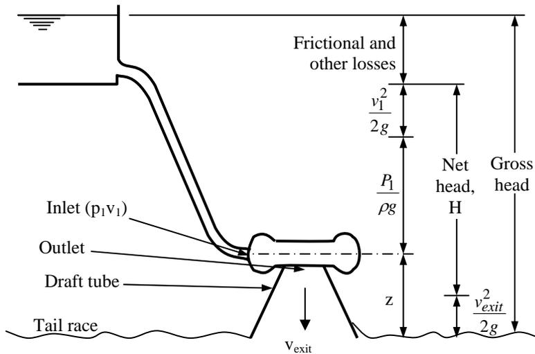
Fig. 1.1: Schematic diagram of a turbine plant.
