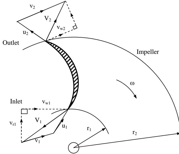
Fig. 4.2: Relative velocity triangles at inlet and outlet.
