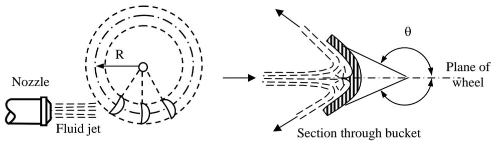
Fig. 3.3: Pelton wheel turbine.
