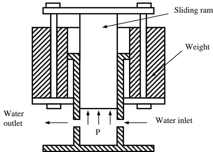
*Fig. 5.5: Hydraulic accumulator*
