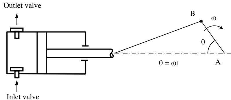
*Fig. 5.1: Piston and cylinder mechanism of reciprocating pump.*
