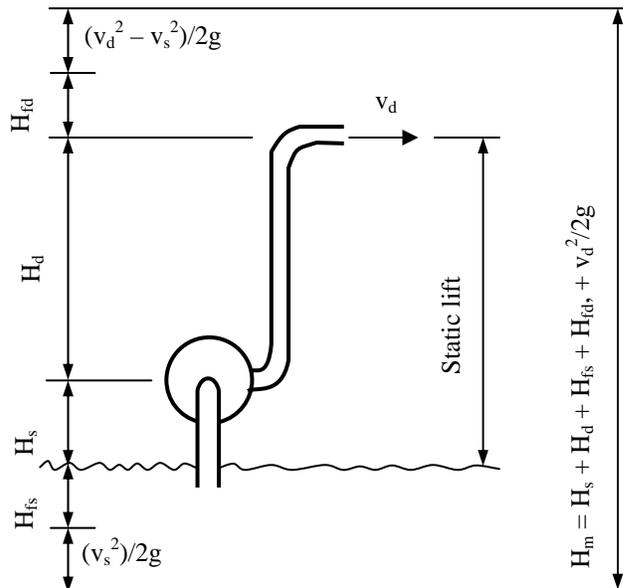
Fig. 4.3: Distribution of the components of manometric head of a pump
