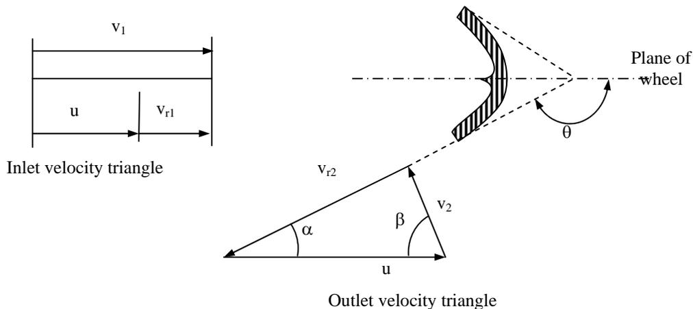
Fig. 3.4: Inlet and outlet velocity triangles.
