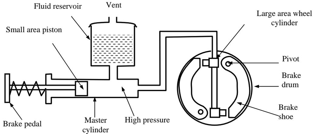
*Fig. 5.7: Hydraulic Vehicle brakes*
