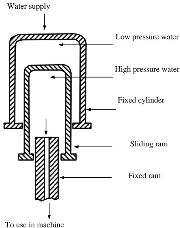
*Fig. 5.6: Hydraulic intensifier*
