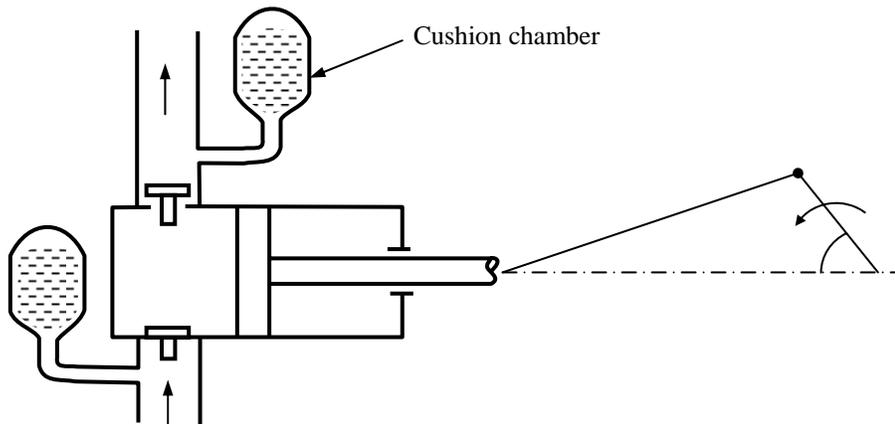
Fig. 5.3: Reciprocating pump fitted with cushion chambers
