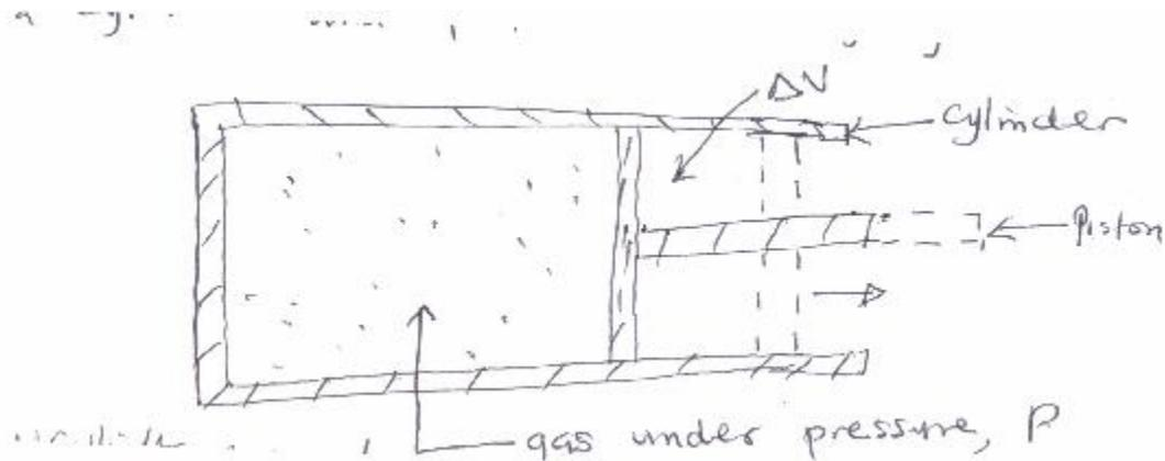
The work ( $dW$ ) done by the gas when the piston moves to the right under pressure  $P$  such that the volume of the gas increases by  $dV$  is
