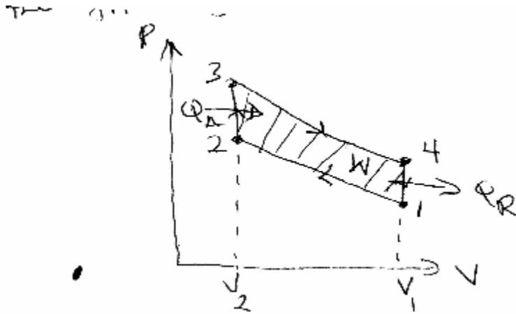
The net work produced by the engine is given by
