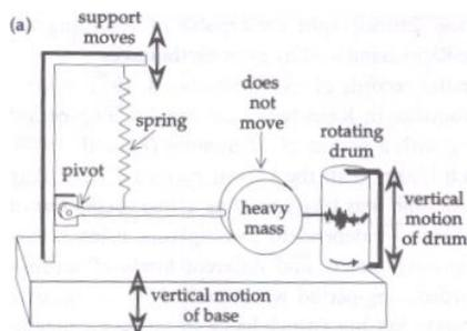
Schematic diagrams illustrating the principle of operation of the vertical-motion seismometer: (a) mechanical pendulum type (after Strahler, 1963), (b) electromagnetic, moving coil type.
