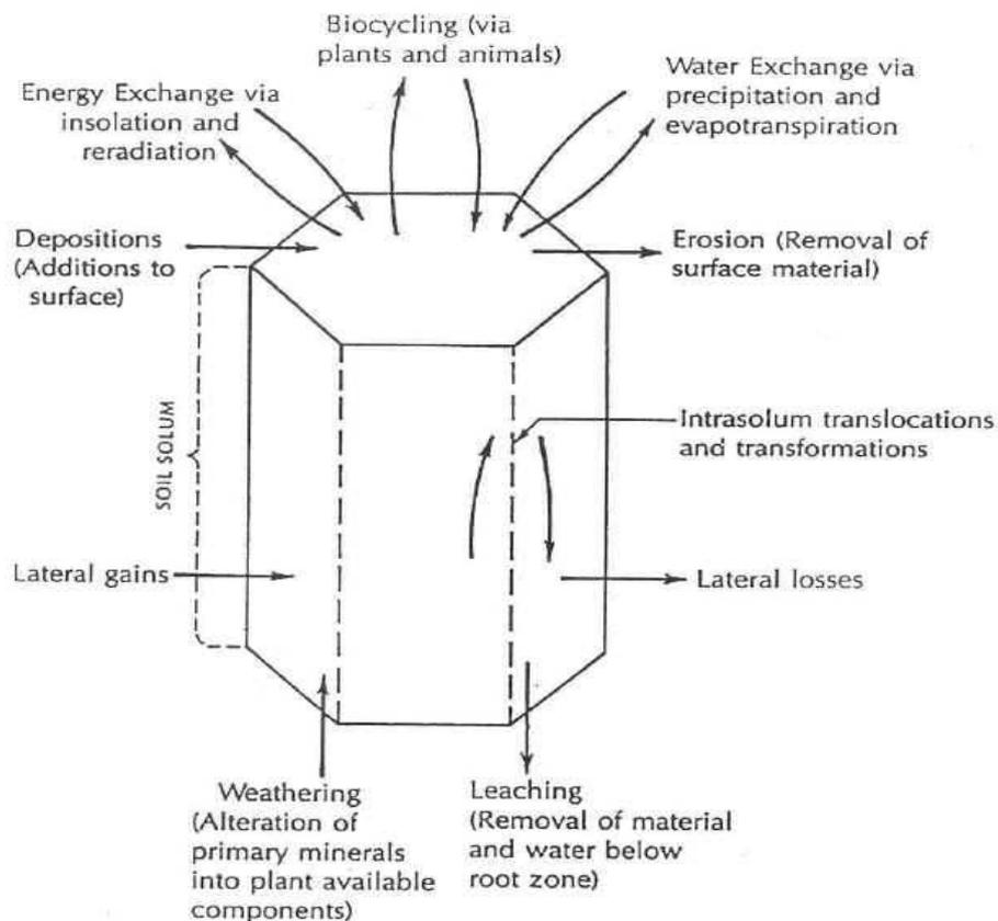
Schematic representation of the solum of a pedon as an open system.
