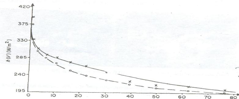
Fig.10. Heat transfer coefficients to a 2.6-mm initial-diameter droplet as a function of droplet volume at  $\Delta T_{mn}$  of 175K. O, theoretical results (Baumeister et al., 1966); x, experimental results.
