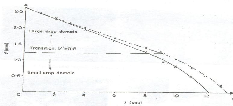
Fig.9: Experimental and theoretical results of changes in drop diameter,  $d$  with elapsed time,  $t$ , for a 2.6-mm initial-diameter droplet and  $\Delta T_{mn} = 175K$ . O, theoretical results, (Baumeister et al., 1966); x, experimental results
