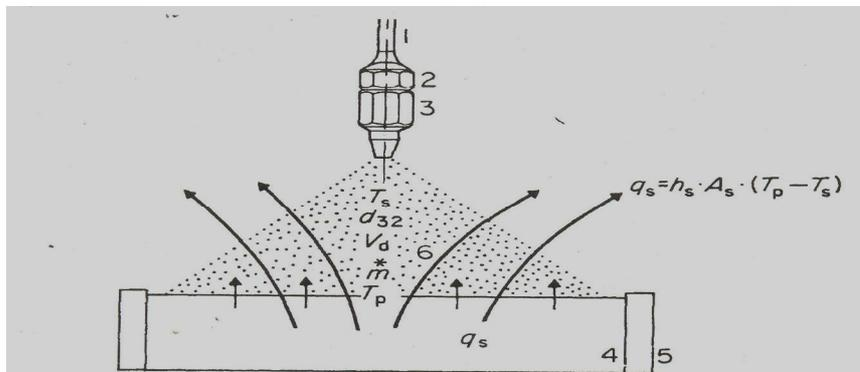
**Fig. 2: Schematic diagram of experimental equipment**
