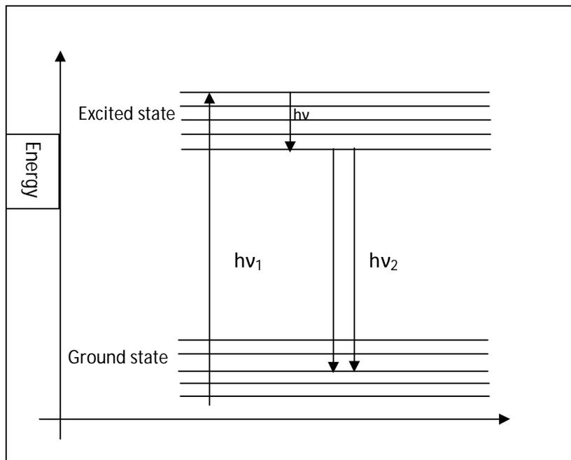
The molecules emit energy  $h\nu$  by collision and drops to the lowest vibrational level of the excited state. The probability of return to ground state with emission of photon is greatest at
