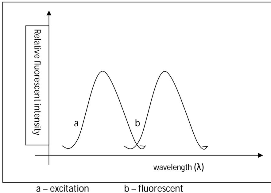
Generally, Beer's law applies to power of radiation transmitted by a substance or solution but modification becomes necessary for fluorescence since radiation is emitted and not transmitted
