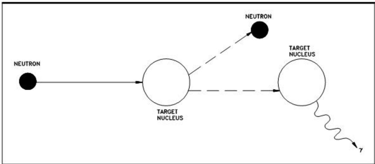
Figure 17 Inelastic Scattering
