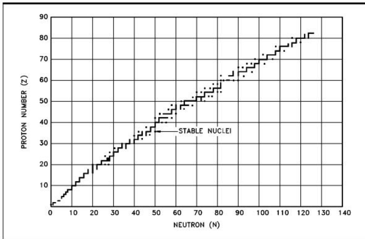
Figure 6 Neutron - Proton Plot of the Stable Nuclides
